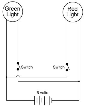
Binary Light Box Wiring Diagram
