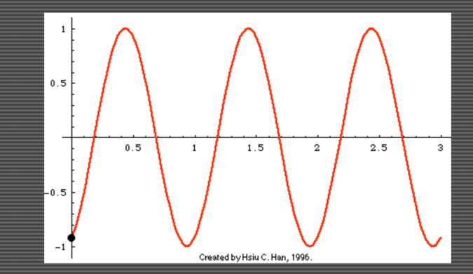
Frequency: the number of times a signal goes through a complete "up and down" cycle in one second of time. 1 Hz
