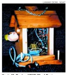
Kevin McCauley, KB3EJM, of East Stroudsburg, Pennsylvania, built the NJ QRP Club PSK Warbler kit into a bird house. The sides are plexiglass so its workings can be seen. Kevin added an AF amp so it "warbles" when in use. The bird on the front of the structure is perched on the AF volume control shaft. Kevin took the "Bird House Warbler" to Field Day, and the Pocono Record, the local newspaper, featured a photograph of this unique PSK transceiver as part of an article on Field Day.
